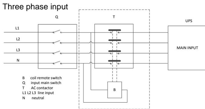
Fig.3-2 Typical external isolating device installation
